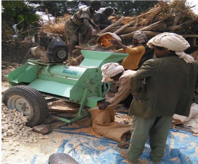
Figure 1. Engine-driven Bako type maize Sheller
